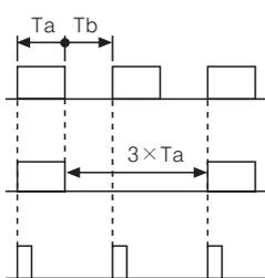
Width of  $T_a$  (ON) and  $T_b$  (OFF) must be larger than Min. signal width.
