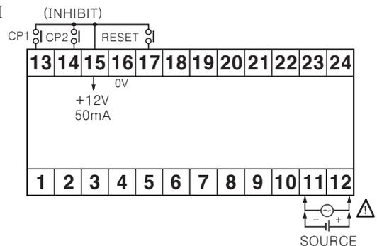
※CP2(INHIBIT) : Time hold terminal when using for timer.
