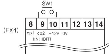
●INHIBIT mode is active when SW1 turns ON. (Time Hold)
