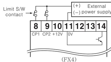
◎Using 2 counters with one sensor
