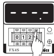
※If pressing one of digital switch buttons ( + , - ) in decimal point setting mode, decimal point will be moved to Up(+) direction.
