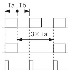
Therefore Ta(ON width) and Tb(OFF width) needed to be over min.signal width.
